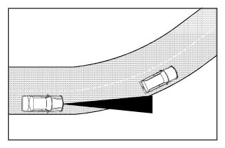
When following a vehicle and entering a curve, Adaptive Cruise Control could lose track of the vehicle in your lane and accelerate your vehicle. When this happens, the vehicle ahead symbol will not appear on the HUD.
